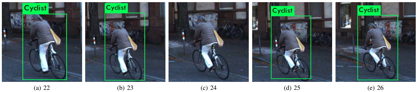
Fig. 3. In session 0005, YOLO intermittently detects the Cyclist with varying levels of probability ( 0 – 75%).
